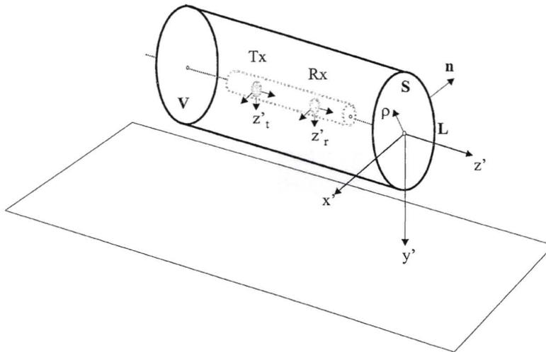
Figure 2: The mathematical model of a horizontal well. A 2-D model's geometry can consist of a set of cylindrical and planar interfaces extended along the  $z'$ -direction. The shape of the cylindrical body is described by volume  $V$ , cross-section area  $S$  and contour of cross-section  $L$ . Vector  $\rho$  is defined at the  $x'y'$ -plane. The tri-axial induction transmitter  $Tx$  and receiver  $Rx$  are located on the  $z'$ -axis at points  $z'_t$  and  $z'_r$ , respectively.
