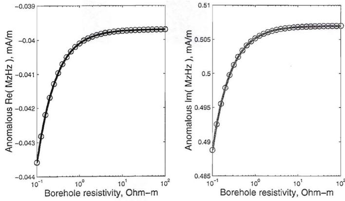
Figure 3: The modeling of a borehole: the comparison between the anomalous magnetic fields calculated by the analytic solution (the solid lines) and nonlinear approximation (the circles).
