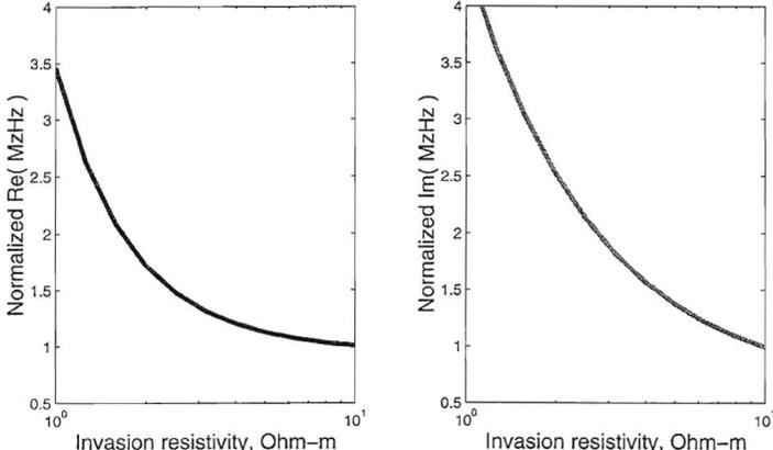
Figure 7: The invaded zone compensation by the 3-coil  $MzHz$  induction tool.
