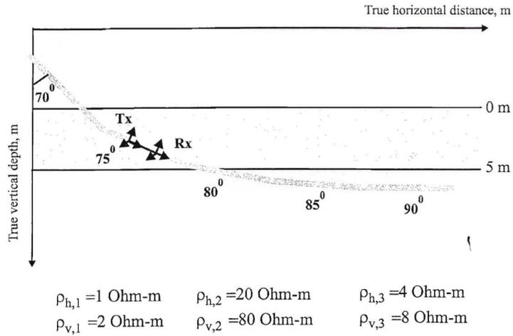
Figure 10: The model of the 3-layer anisotropic formation and directional well of varying dipping angle.
