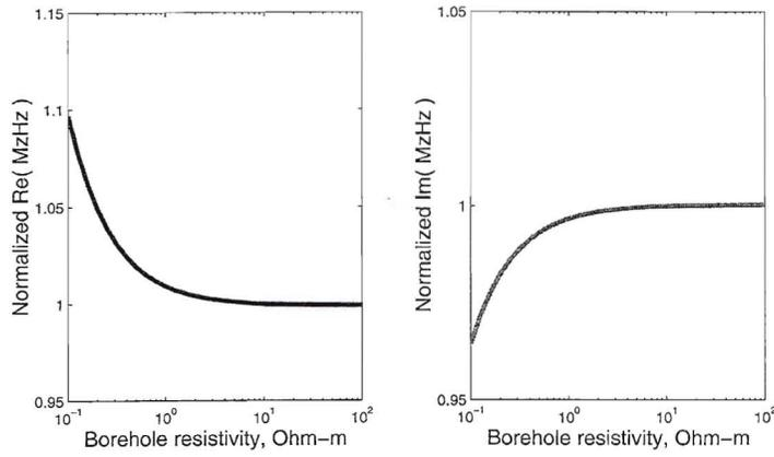
Figure 4: Borehole compensation with the 3-coil *MzHz* induction tool.
