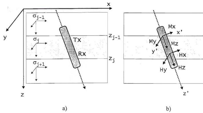
Figure 9: The tensor induction tool in a layered anisotropic formation: the model coordinate system  $\{x, y, z\}$  (a) and the instrument coordinate system  $\{x', y', z'\}$ .
