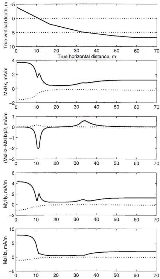
Figure 13: The tensor logs in the subhorizontal well with varying dipping angles. The top frame shows the trajectory and the locations of the formation boundaries. The four frames below demonstrate the tool responses for the tool component configurations  $MxHx$ ,  $(MxHz - MzHx)/2$ ,  $MyHy$ , and  $MzHz$ . The in-phase and quadrature parts of the magnetic field are shown by the dashed and solid lines, respectively. The magnetic field in air is subtracted from the total signals.
