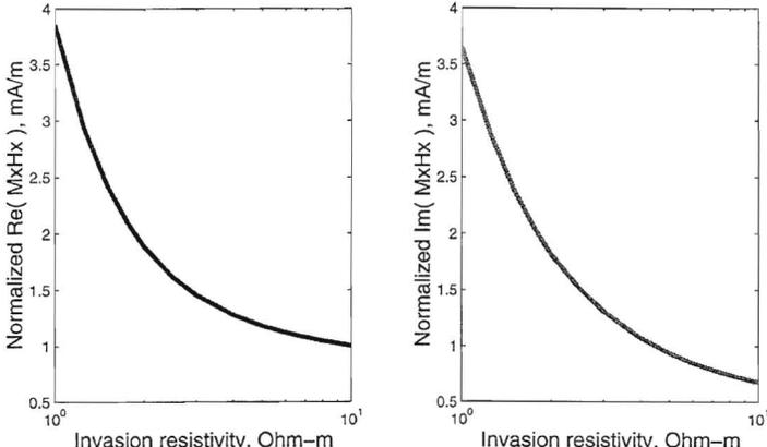
Figure 8: The invaded zone compensation by the 3-coil  $MxHx$  induction tool.
