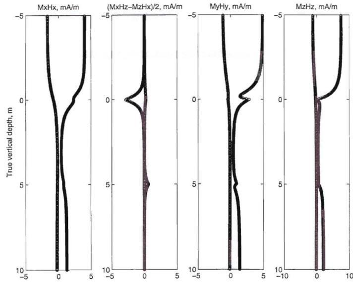
Figure 12: The tensor logs in the 3-layer anisotropic model and deviated well of 85°. The two parts of the magnetic field (the in-phase and quadrature components) are calculated by using the code for a deviated well (the dotted and solid lines) and the code for a horizontal well (the circles).
