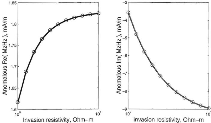
Figure 6: The modeling of an invaded zone: the comparison between the anomalous magnetic fields calculated by the analytic solution (the solid lines) and nonlinear approximation (the circles).
