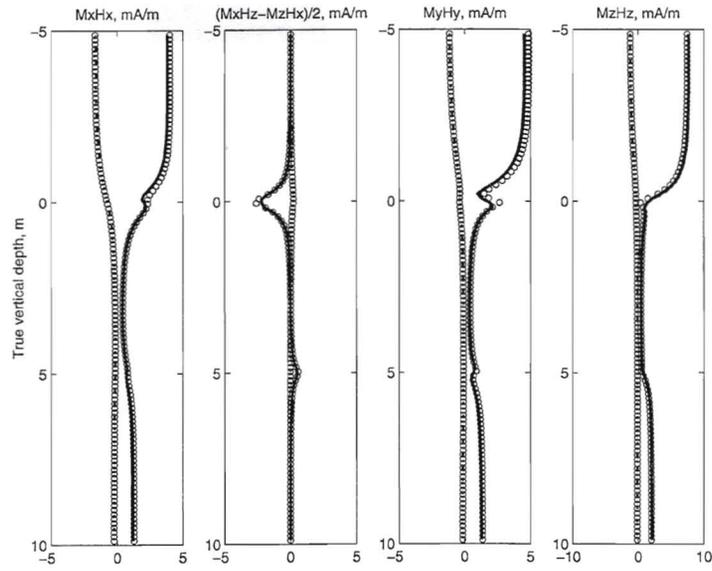
Figure 11: The tensor logs in the 3-layer anisotropic model and deviated well of 75°. The two parts of the magnetic field (the in-phase and quadrature components) are calculated by using the code for a deviated well (the dotted and solid lines) and the code for a horizontal well (the circles).
