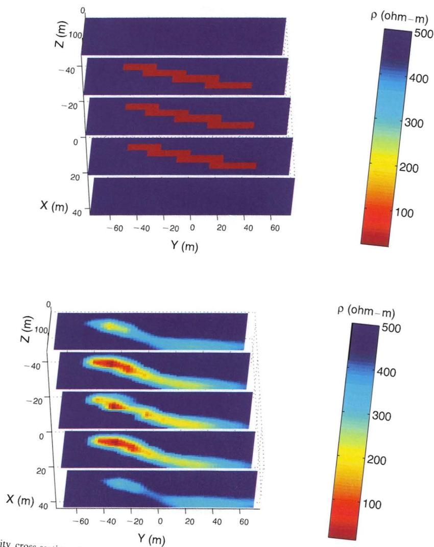
Figure 8. Successive resistivity cross-sections through the 3-D geoelectric model of a conductive, dipping dike in a homogeneous half-space (top panel), and the corresponding LQL inversion result (bottom panel).
