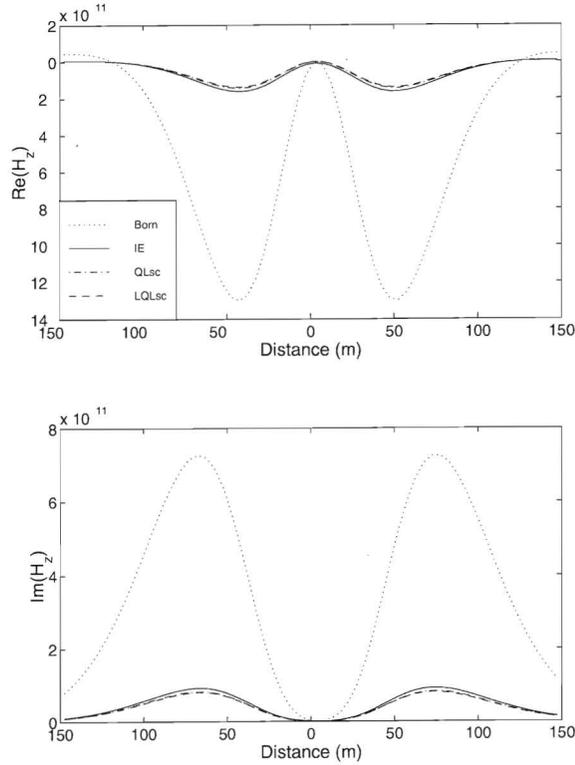
**Figure 4.** Numerical comparison of full IE solution (IE), Born approximation (Born), scalar QL approximation (QLsc), and scalar LQL approximation (LQLsc) at frequency  $f=56$  kHz for Model 2 (Fig. 3). The real and imaginary parts of the vertical component of the anomalous magnetic field are presented at receivers along the  $Y$ -axis at a height of 30 m above the ground.
