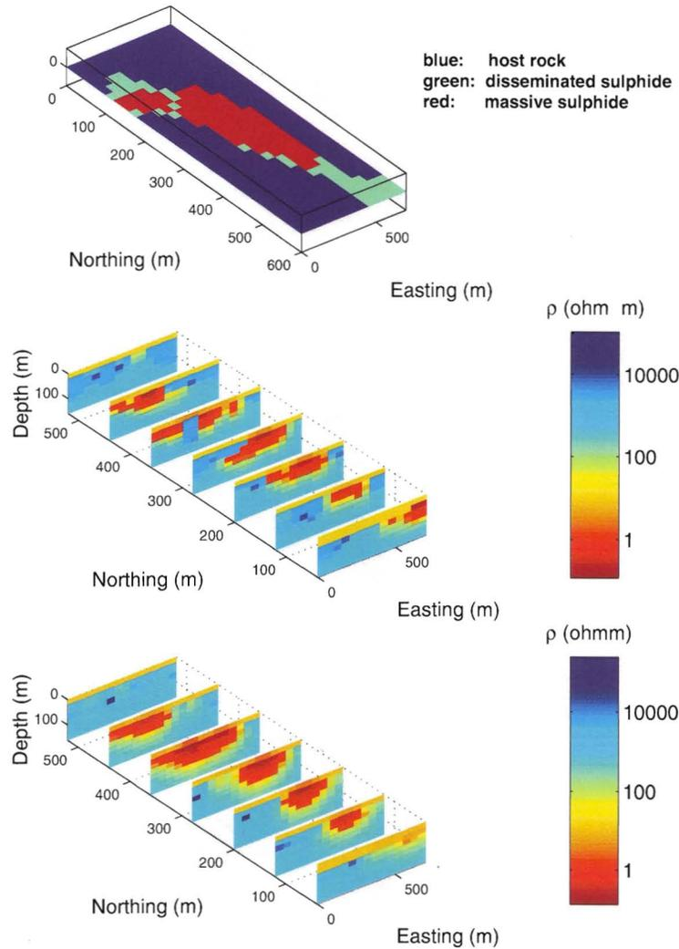
**Figure 14.** Horizontal extent of the sulphides in the inverted area as inferred from Fig. 11 (top panel), and cross-sections of the inverted volume for the coplanar (middle panel) and the coaxial (bottom panel) components.
