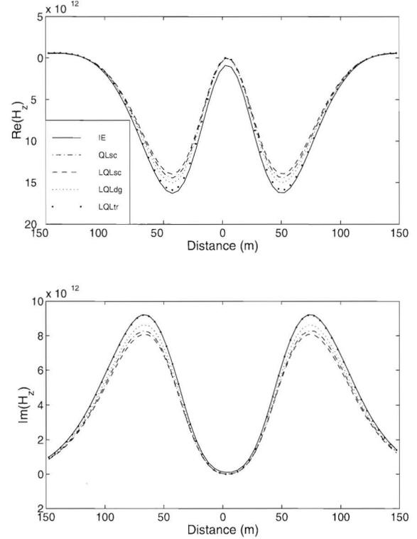
**Figure 5.** Numerical comparison of full IE solution (IE), scalar QL approximation (QLsc), scalar LQL approximation (LQLsc), diagonal LQL approximation (LQLdg) and tensor LQL approximation (LQLtr), at frequency  $f=56$  kHz for Model 2 (Fig. 3). The real and imaginary parts of the vertical component of the anomalous magnetic field are presented at receivers along the  $Y$ -axis at a height of 30 m above the ground.
