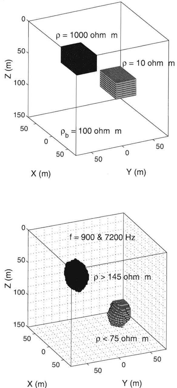
Figure 10. Model 4: 3-D geoelectric model of one conductive and one resistive rectangular inclusion in a homogeneous half-space (top panel), and 3-D image of the LQL inversion result (bottom panel).
