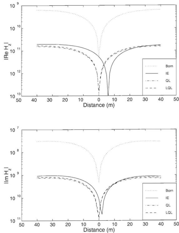
Figure 2. Numerical comparison of the full IE solution, Born approximation, scalar QL approximation, and scalar LQL approximation at frequency  $f=100$  Hz for Model 1 (Fig. 1). Absolute values of the real and imaginary parts of the anomalous magnetic field are presented at receivers on the surface along the  $Y$ -axis.
