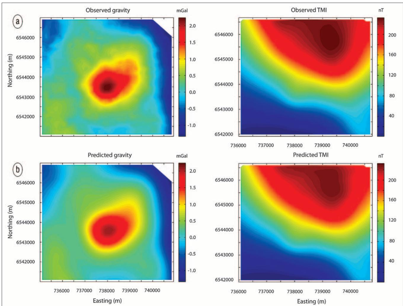
**Figure 3.** Observed (a) and predicted (b) surface-based gravity (left panels) and airborne TMI (right panels) from the 3D joint inversion of the Carrapateena IOCG deposit. The weighted misfit between observed and predicted data is less than 2%.
