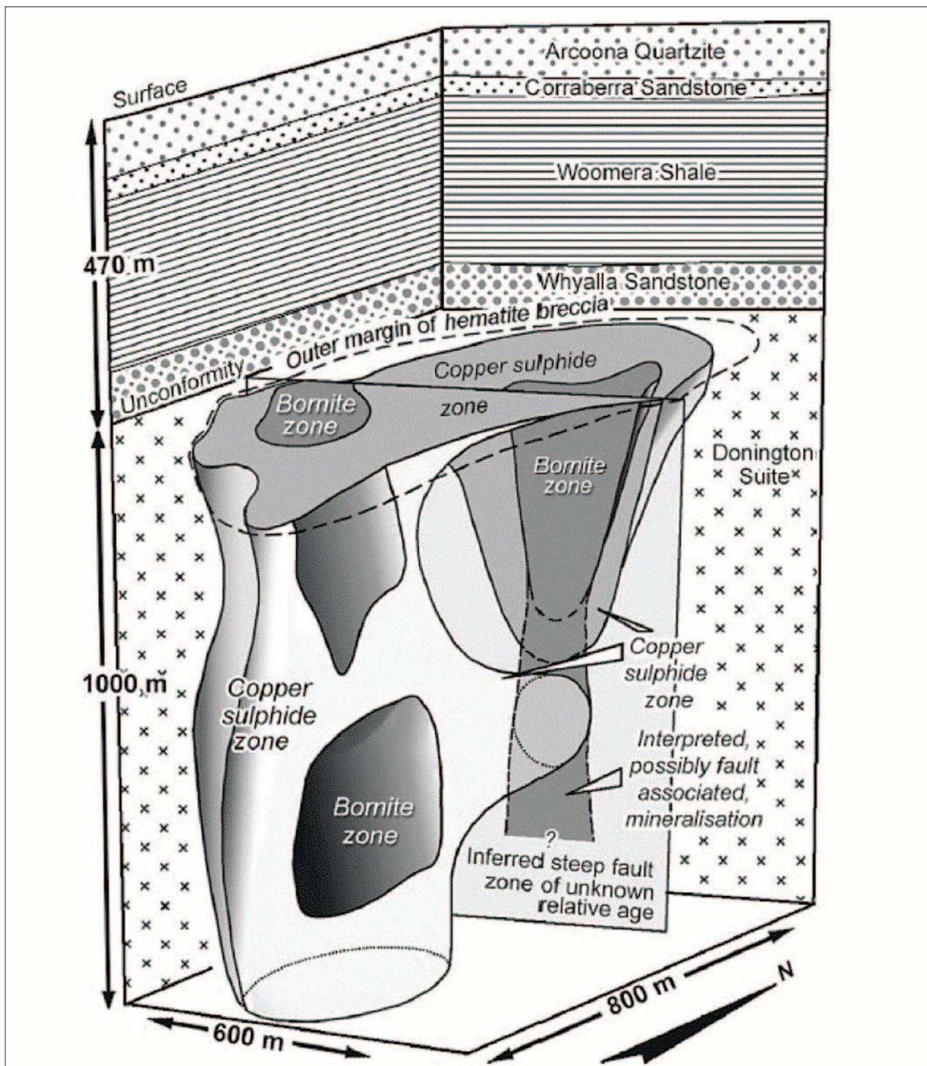
Figure 2. Cartoon of the geology of the Carrapateena IOCG deposit, located beneath Stuart Shelf sediments (courtesy of PIRSA).
