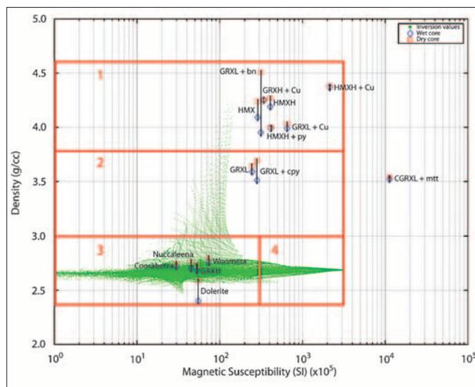
**Figure 4.** Crossplot of the density and susceptibility values for all cells in the 3D Earth model (green dots) as recovered from joint inversion superimposed on the laboratory-based density and susceptibility measurements of drill core samples from Vella and Emerson (2009). The abbreviations for different lithologies are consistent with Vella and Emerson (2009). Groups have been assigned on the basis of their physical properties.
