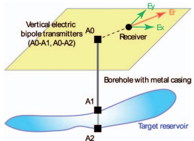
Figure 3 Sketch of typical BSEM survey configuration.
