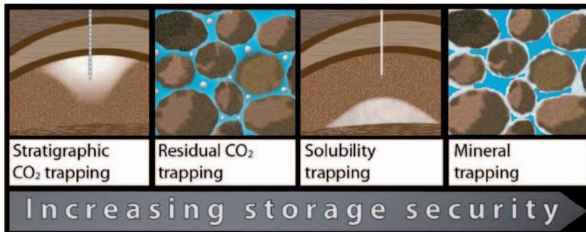
Figure 1 Conceptual sketch of the different mechanisms of CO<sub>2</sub> trapping.
