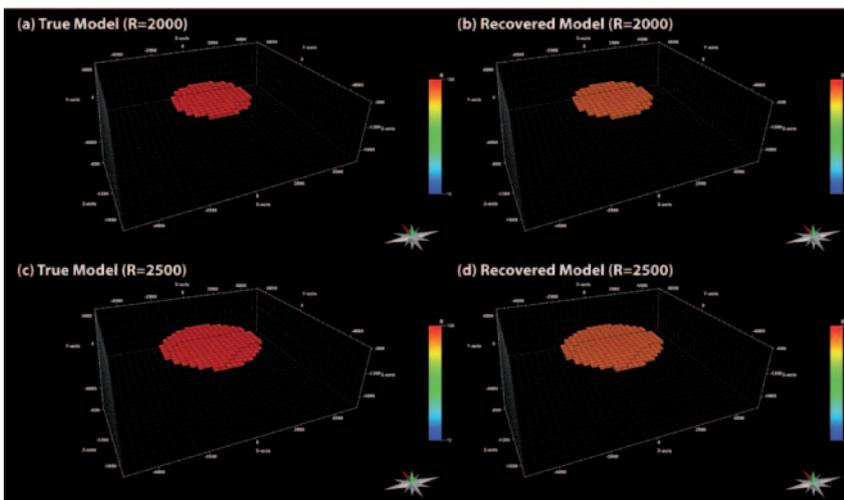
Figure 10 3D perspective view of the true model of CO<sub>2</sub> plume and the image recovered from 3D inversion of BSEM data (R = 2000 and 2500 m).
