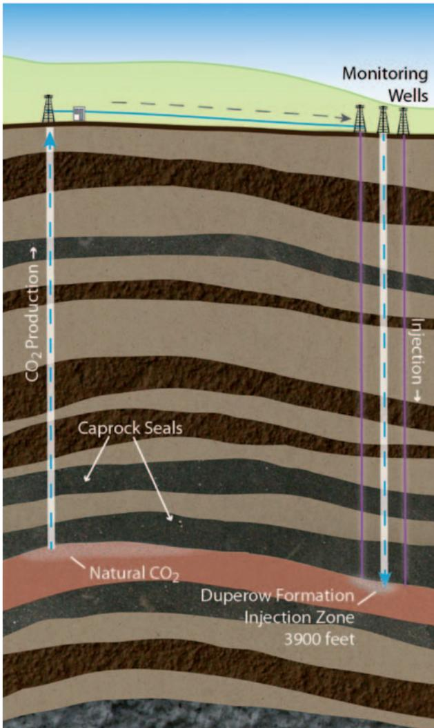
Figure 5 Schematic view of the Kevin Dome project.
