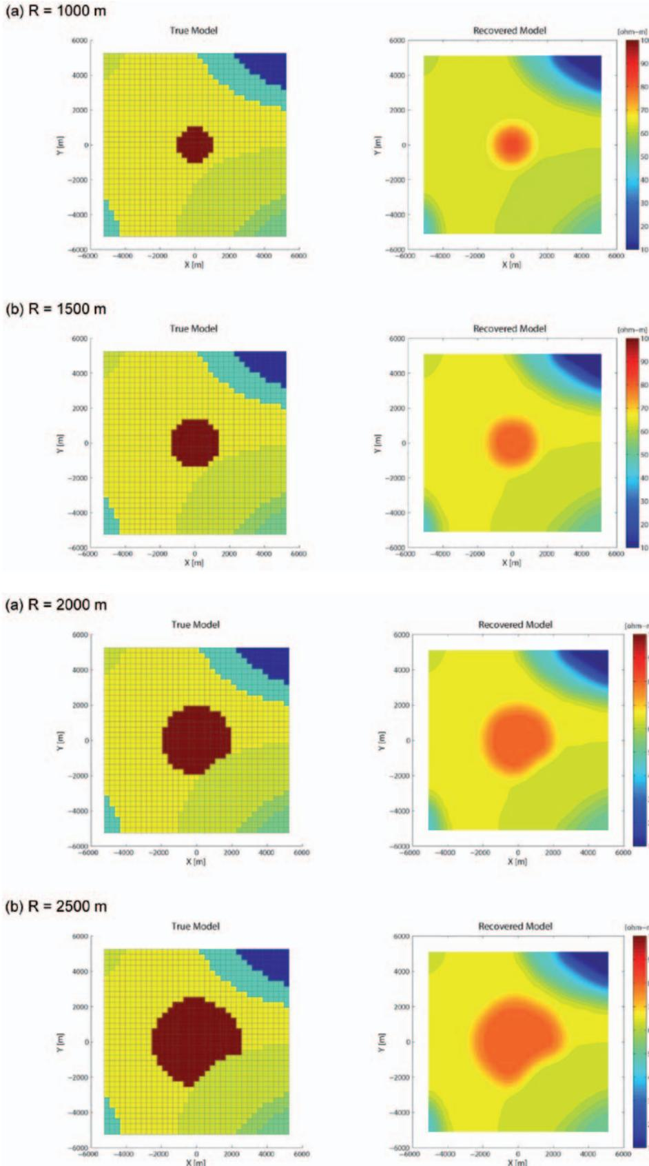
Figure 11 Comparison between the true resistivity model and the inverse model at the same depth of 1125 m for different stages of CO<sub>2</sub> sequestration (R = 1000 and 1500 m).
