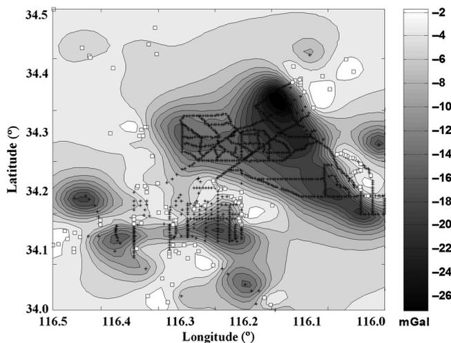
Figure 12. Isostatic Bouguer gravity grid after removal of the bedrock component.
