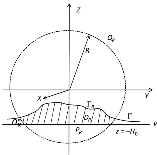
Figure 1. Density contrast model for a sediment-basement interface with a positive anomaly. The horizontal plane  $P$  is located at the average depth of the sediment-basement interface, and  $\Gamma_R$  is the actual sediment-basement interface.
