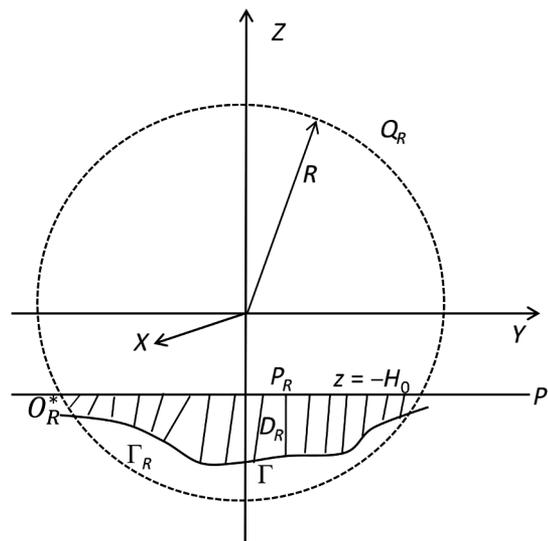
Figure 2. Density contrast model for a sediment-basement interface with a negative anomaly. The horizontal plane  $P$  is located at the average depth of the sediment-basement interface, and  $\Gamma_R$  is the actual sediment-basement interface.
