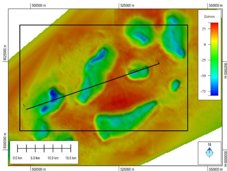
**Figure 1** Map of the observed  $G_{zz}$  component of gravity gradiometry data used in the inversion. The black box outlines the inversion domain. The black line labeled LL' indicates the location of the vertical sections.
