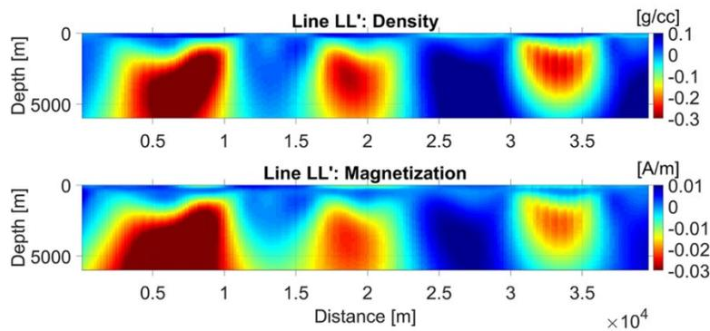
**Figure 3** Vertical sections extracted from the joint probabilistic Gramian inversion along profile LL'. I. The top panel shows the anomalous density. The bottom panel shows the induced magnetization projected onto the inducing field.
