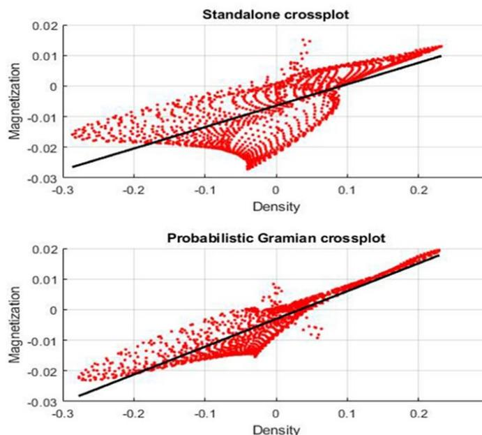
**Figure 4** Model parameter cross plot comparison of the different inversion methodologies. The top panel shows the correlation of the standalone inversions. The bottom panel shows the correlation of the probabilistic Gramian inversion.
