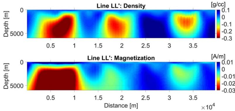
**Figure 2** Vertical sections extracted from the standalone inversions along profile LL'. The top panel shows the anomalous density. The bottom panel shows the induced magnetization projected onto the inducing field.
