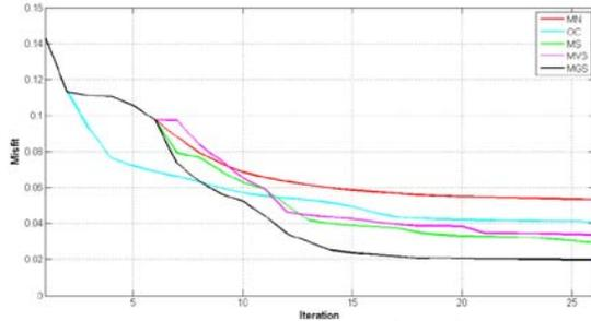
**Figure 4.** Convergence of the misfit for the following stabilizers: Occam (OC), minimum norm (MN), minimum support (MS), minimum vertical support (MVS), and minimum gradient support (MGS). These convergence plots are shown for the iterative migration of the inline electric field only.
