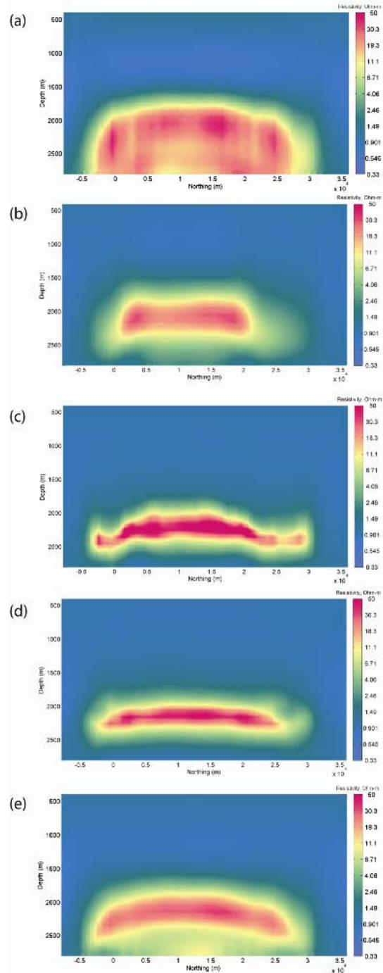
**Figure 5.** Resistivity cross-sections obtained using (a) Occam, (b) minimum norm, (c) minimum support, (d) minimum vertical support, and (e) minimum gradient support stabilizers for migration of the inline electric field.
