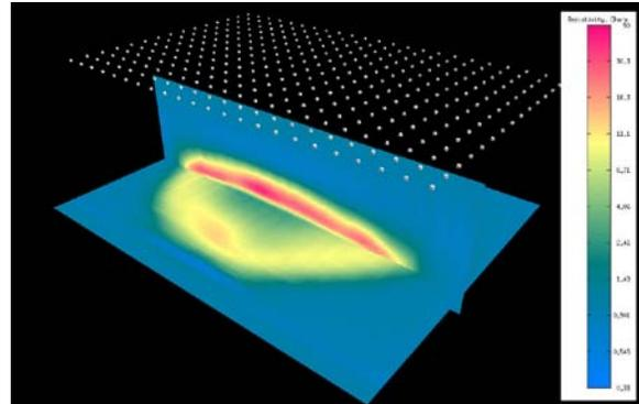
**Figure 3.** 3D view of the Shtokman resistivity model obtained from the joint iterative migration of the inline and vertical electric and transverse magnetic fields using the MGS stabilizer. The sections correspond to those shown in Figure 2. A vertical exaggeration of 6 was used in this image.
