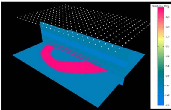
**Figure 2.** 3D view of the Shtokman resistivity model, with three of the four reservoir units shown. The vertical section corresponds to those vertical cross-sections shown in subsequent figures. The horizontal section shows the extent of the main reservoir unit. Receiver positions are denoted by the grey cubes. A vertical exaggeration of 6 was used in this image.
