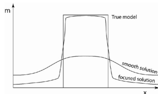
**Figure 1.** A smooth stabilizer will recover a model with a smooth distribution of model parameters. A focusing stabilizer will recover a model with sharper boundaries and contrasts, and will be closer to the true model.
