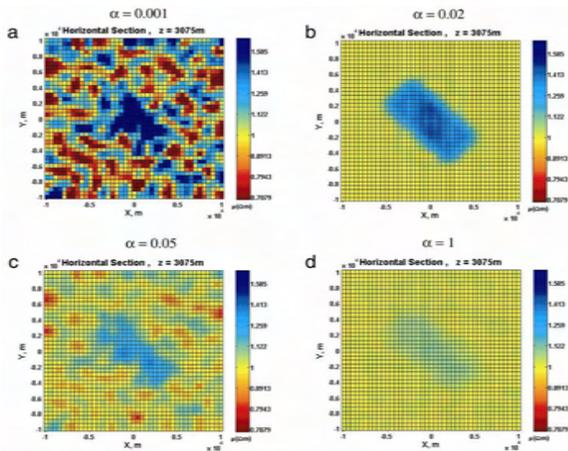
Figure 6: Model 1. A horizontal cross-section of the 3-D smooth inversion result at a depth of 3075 m for different values of the  $\alpha$ .
