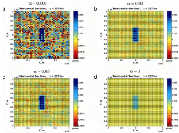
Figure 5: Model 1. A horizontal cross-section of the 3-D smooth inversion result at a depth of 2275 m for different values of the  $\alpha$ .
