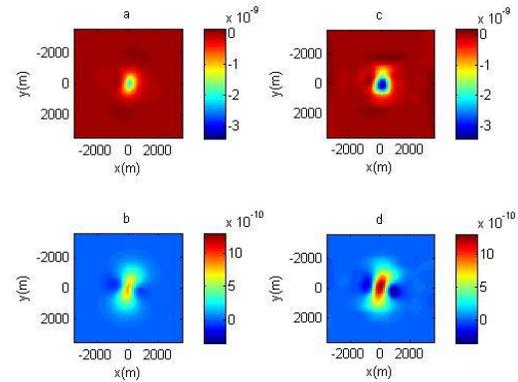
**Figure 8.** A comparison between the real (upper panels) and imaginary (lower panels) components of the  $x$ -directed electric field on a plane  $P$  located at 500 meters below the earth's surface  $\Sigma$  computed using IE modeling (left panels) and by the Stratton-Chu integral transform (right panels).
