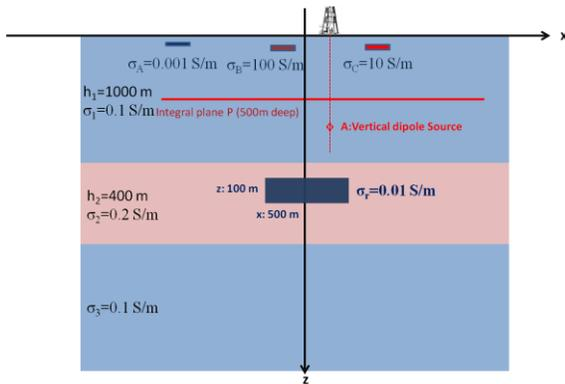
**Figure 7.** Vertical cross section of the reservoir target embedded in a layered host with near-surface inhomogeneities. The actual and virtual receiver profiles are shown, along with the borehole and BSEM transmitter location.
