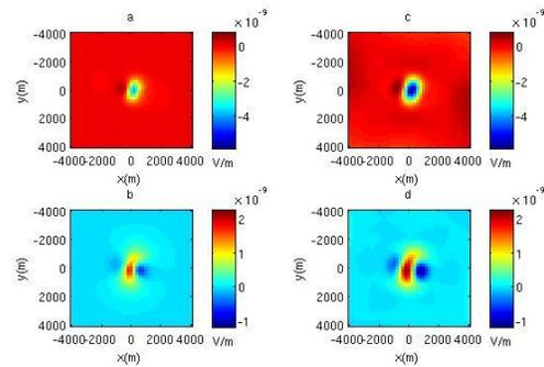
**Figure 5.** A comparison between the real (upper panels) and imaginary (lower panels) components of the  $x$ -directed electric field on a plane  $P$  located at 500 meters below the earth's surface  $\Sigma$  computed using IE modeling (left panels) and by the Stratton-Chu integral transform (right panels).
