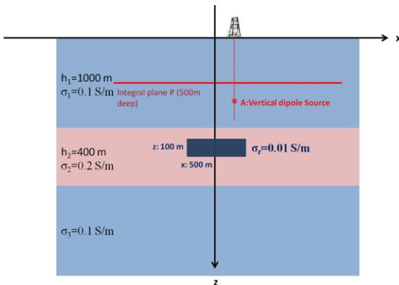
**Figure 3.** Vertical cross section of the reservoir target embedded in a layered host. The actual and virtual receiver profiles are shown, along with the borehole and BSEM transmitter location.
