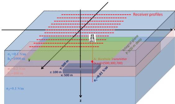
**Figure 2.** 3D perspective view of the reservoir target embedded in a layered host. The actual and virtual receiver profiles are shown, along with the borehole and BSEM transmitter location.
