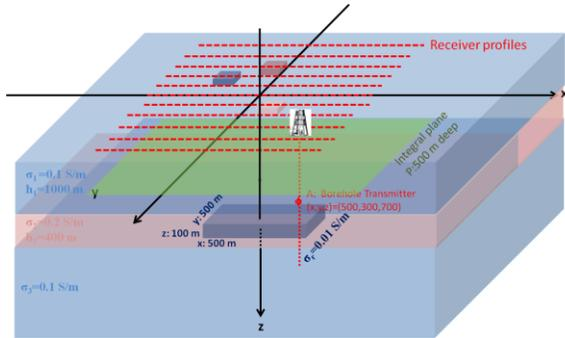
**Figure 6.** 3D perspective view of the reservoir target embedded in a layered host with near-surface inhomogeneities. The actual and virtual receiver profiles are shown, along with the borehole and BSEM transmitter location.
