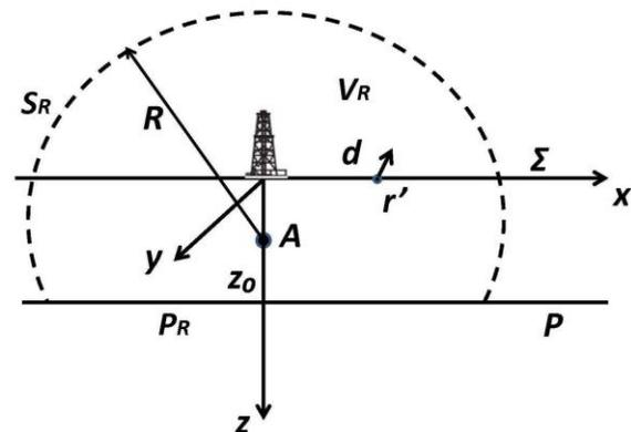
Figure 1. A model of a typical BSEM survey with the transmitter  $T_A$  located at some point  $A$  within the borehole and the receivers distributed over the earth's surface  $\Sigma$  with the radius vector  $\mathbf{r}'$ .
