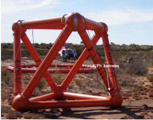
Figure 2. A second set of AirMt coils are used for the reference station.
