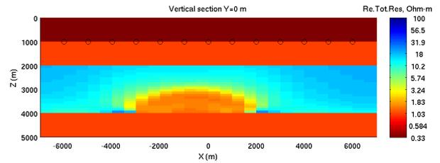
Figure 4: The vertical section through the result of the conventional inversion of MT data.
