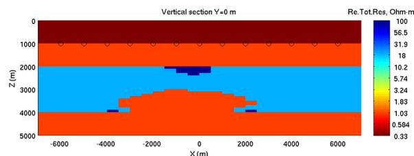
Figure 9: The vertical section through the result of the multinary joint inversion of MCSEM and MT data.
