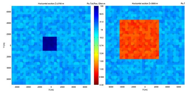
Figure 3: Horizontal sections of true Model 1. A 2700 m depth section is shown on the left and 3900 m is shown on the right. Receivers are shown by circles.
