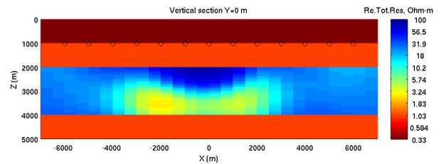
Figure 5: The vertical section through the result of the conventional inversion of MCSEM data.
