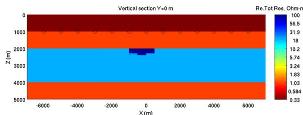
Figure 8: The vertical section through the result of the multinary inversion of MCSEM data.
