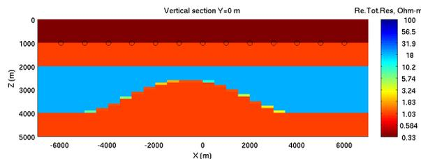
Figure 7: The vertical section through the result of the multinary inversion of MT data.
