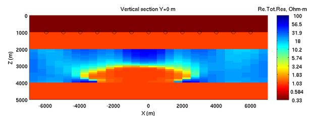
Figure 6: The vertical section through the result of the conventional joint inversion of MCSEM and MT data.
