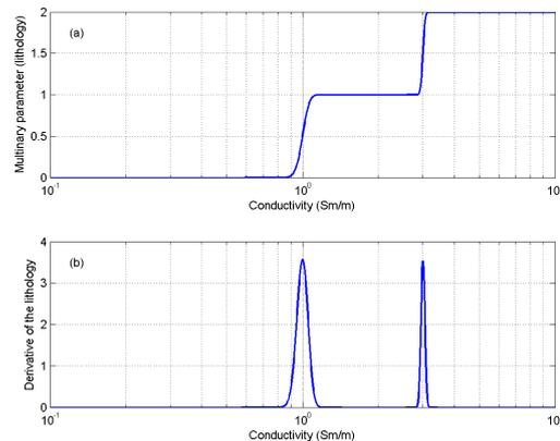
Figure 1: (a) - An example of transformation of the conductivity into multinary parameters. (b) - Derivative of the multinary function.
