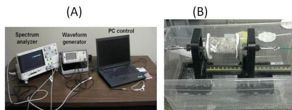
**Figure 2.** Complex resistivity measurement system consisting of waveform generator, spectrum analyzer, PC control (A), and rock sample holder (B).
