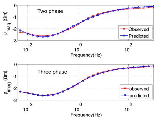
**Figure 4.** The complex resistivity (CR) spectra (red lines) and the data predicted based on the GEMTIP model (blue lines) for sample #8. The top panel presents the result for the two phase GEMTIP model; the bottom panel shows the result for the three-phase GEMTIP model.
