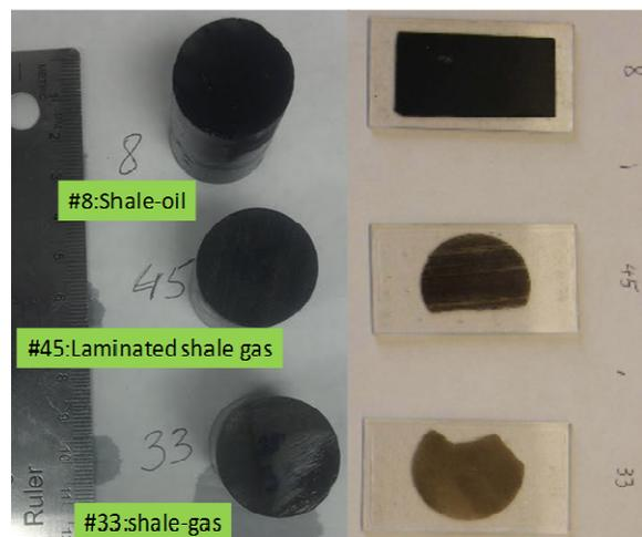
**Figure 1.** The left panels: photos of three shale samples. The right panels: thin sections of the same rock samples prepared for QEMSCAN analysis.
