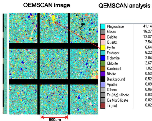
**Figure 3.** The QEMSCAN image of shale oil on the left with a phase analysis on the right. The arrow show example of pyrite in this sample.
