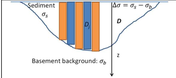
Figure 1: A sketch of a conductivity model of the sedimentary basin. Domain  $D$  represents the conductive sediments with conductivity  $\sigma_s$ , which is discretized into a grid of vertical columns.
