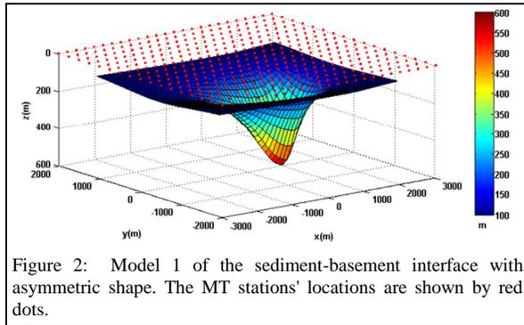
Figure 2: Model 1 of the sediment-basement interface with asymmetric shape. The MT stations' locations are shown by red dots.
