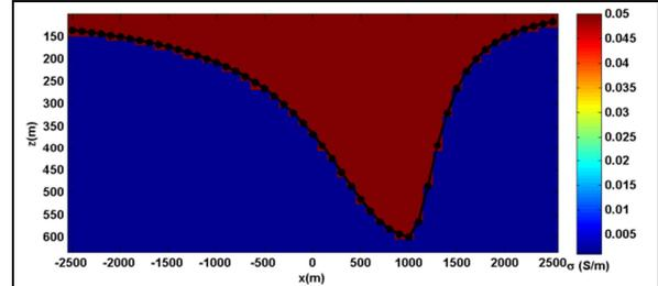
Figure 3: A vertical cross section at  $y=0$  of Model 1 of the sediment-basement interface with asymmetric shape. The black line indicates the actual sediment-basement interface, while the prismatic approximation of the interface is shown by the dark red color, reflecting the conductivity of the sediments of 0.05 S/m on the corresponding color scale.
