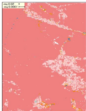
Figure 2. A QEMScan image of the rock sample #37 from Au-Cu deposit. The calcite and quartz are designated by dark and light pink colors, respectively, while dolomite is shown by blue, chalcopyrite by orange, and pyrite by yellow in this image.
