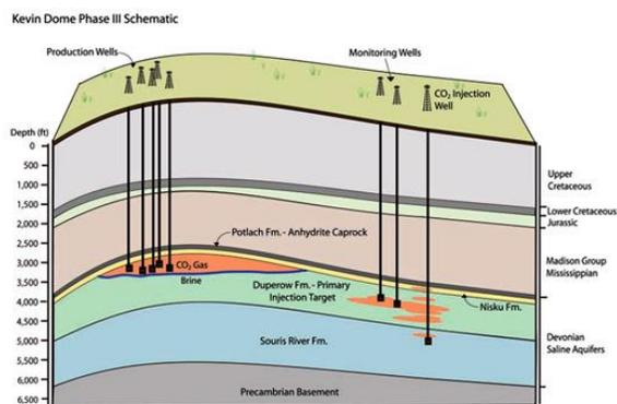
Figure 2: Schematic view of the Kevin Dome project.
