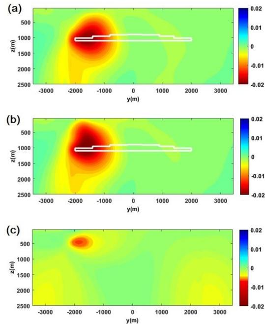
Figure 8: Comparison of the migration images for the leakage model at the 25% gas-injected stage: (a) no leakage; (b) with leakage; (c) difference between the two images.
