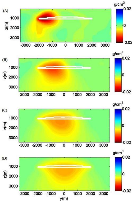
Figure 5: Images produced by the migration of the fields calculated as the differences between the data observed at the current stage of CO<sub>2</sub> injection and at the initial stage before the start of the injection.
